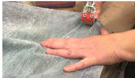
Deborah uses a range of surprising tools to distress garments. Here she uses a rasp that is usually used to give shoes traction.
